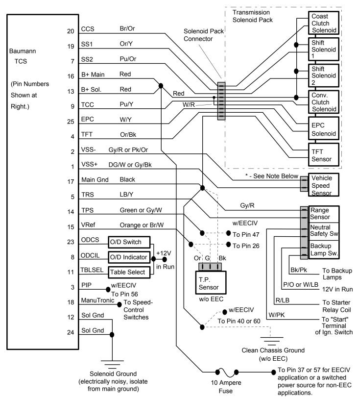
\* - Note: Connect VSS inputs to speedometer outputs on 1992 and later trucks with Rear ABS and electronic speedometer.
