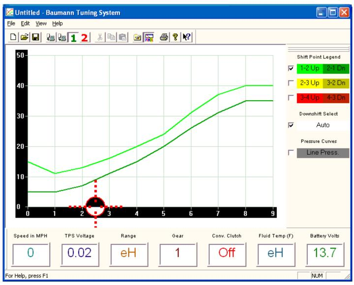
The main window is where all of the shift point and line pressure editing is done. It also serves as the control center from which to load and save data files and to write or read a data file from the permanent calibration memory in the TCS unit.
